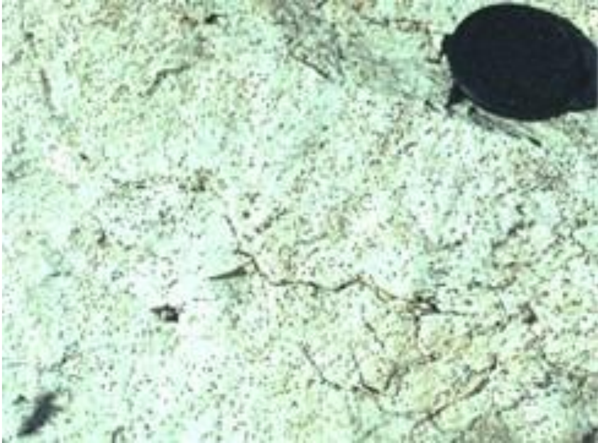
Figure 4. Gold Butte leucogranite consisting of tiny garnet crystals in a matrix of sodic plagioclase, quartz, and trace K-feldspar. (Camera lens cap for scale)
