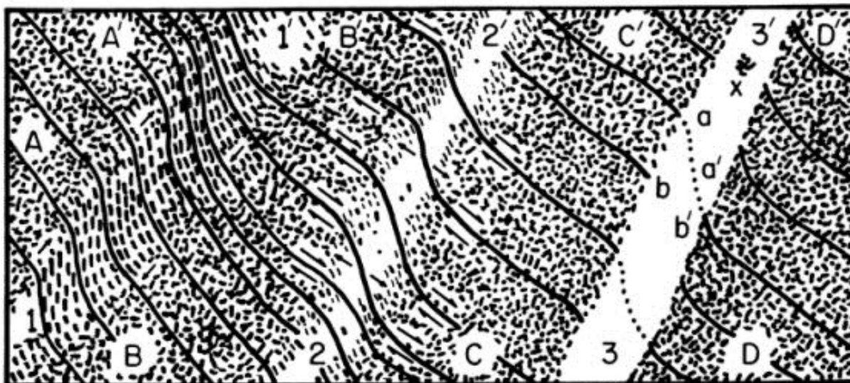
Fig. 5. Diagram showing theoretical stages in the formation of aplite and pegmatite dikes that replace diorite-gabbro wall rock. Areas between A-A', B-B', C-C', and D-D' represent the original massive diorite-gabbro with randomly oriented crystals. Area between 1-1' represents flexed rock in which shearing and cataclasis have oriented the crystals into parallel or subparallel alignment. Here the ferromagnesian silicates are partially replaced by quartz. Area between 2-2' shows differential movements parallel to foliation, which produce relatively low-pressure sites into which silica can move to replace the ferromagnesian silicates by quartz and into which K can move to replace zoned plagioclase to form microcline, myrmekite, and unzoned plagioclase. Migmatite can occur on either side of the 'dike,' but a central zone, where replacement is complete, is aplite or pegmatite. Remnant dark minerals show traces of the former flexed foliation. Area between 3-3' shows an aplite-pegmatite dike cutting across massive diorite-gabbro wall rock. A faint foliation is truncated by the granitic dike; layer b-b' appears to match up, however, a-a' actually connects equivalent layers. Island x is a remnant block of unshered massive diorite-gabbro which remained as an enclave in the dike.
