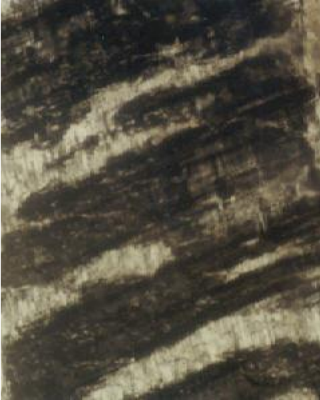
Fig. 12. Vein perthite with albite lamellae (light gray) in microcline (dark gray; grid-twinned), formed by exsolution processes in pegmatite.
