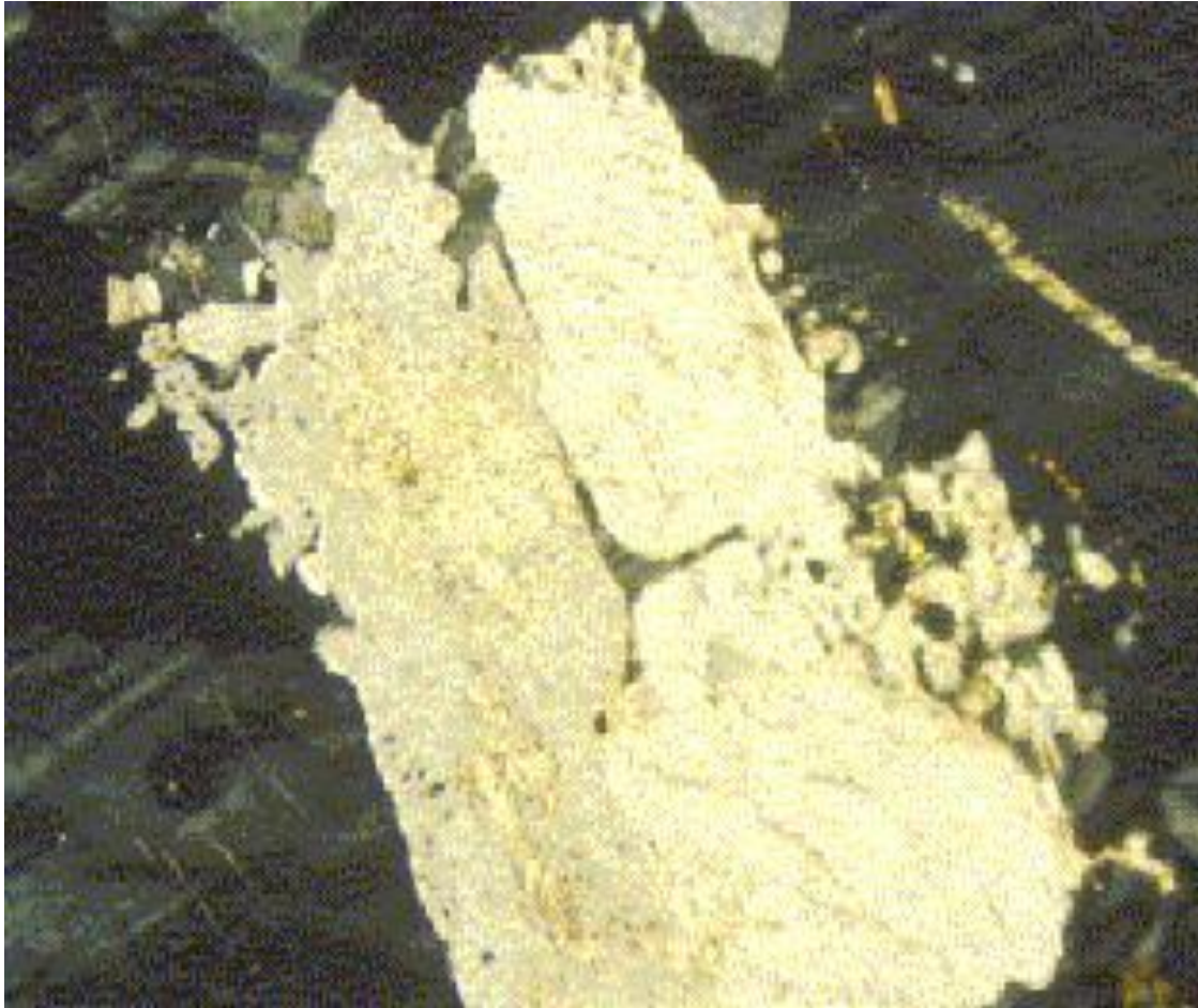
Fig. 15. Interior replacement of plagioclase (white) by veins of microcline (dark gray, black) and islands of unreplaced plagioclase in adjacent microcline. The islands have optically parallel continuity with the larger unreplaced plagioclase grain. Sample obtained from center of the middle part of the Fowler granite body.
