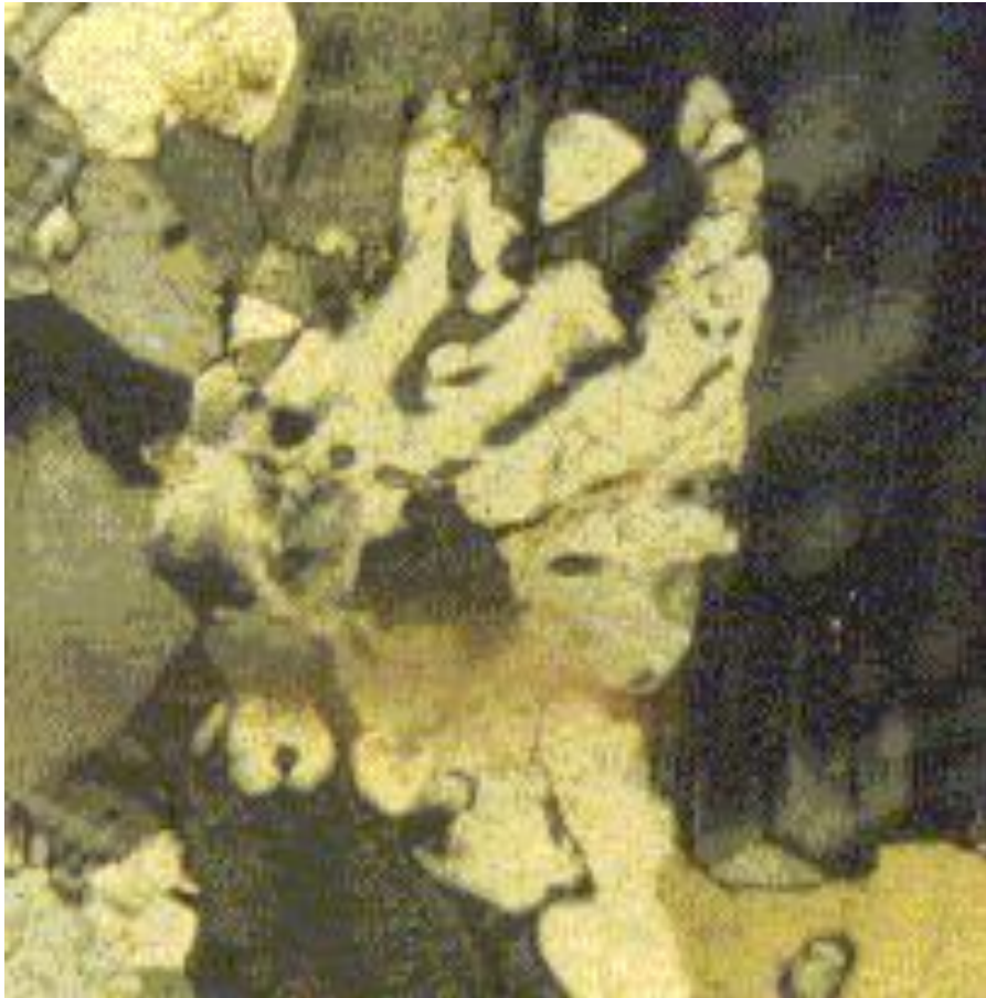
Fig. 10. Veins of microcline (black, dark gray; grid-twinning) replacing interiors of plagioclase (light cream-gray). Remnant islands of unreplaced plagioclase (light gray) occur in the microcline. Sample obtained from southeastern part of Gray's School granite body.
