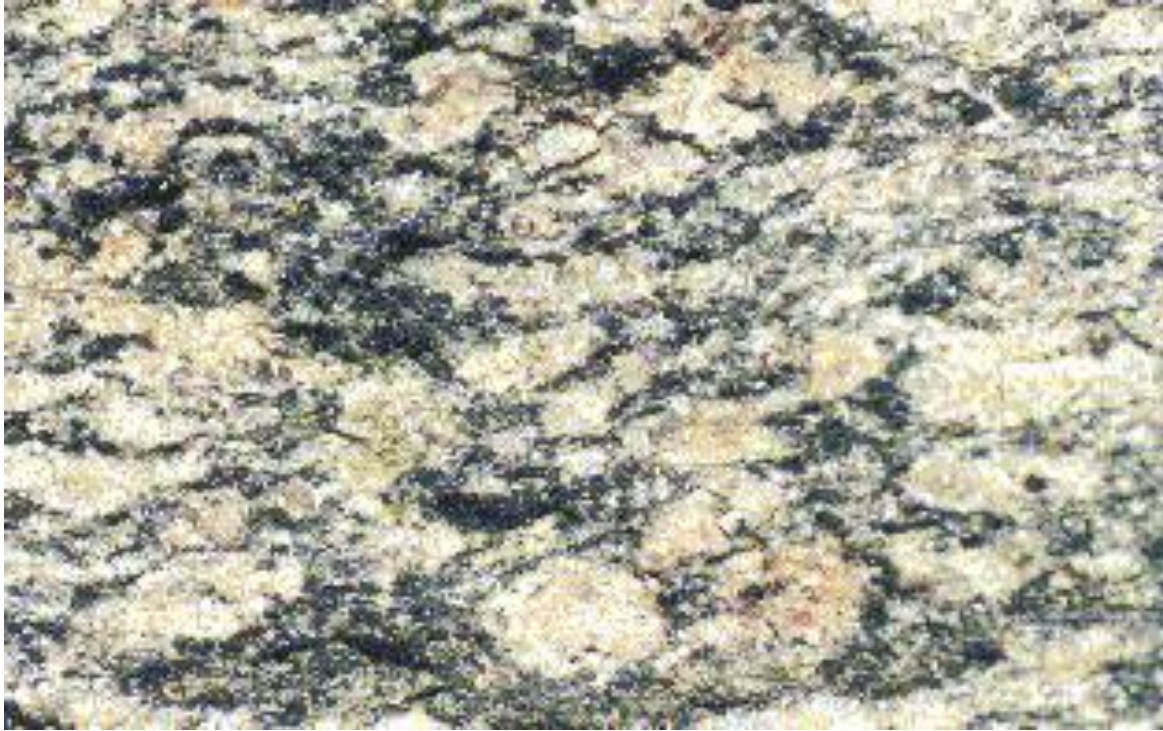
Fig. 8. Megacrystal Gray's School granite along Old River Road. Largest microcline megacrysts (light pink) are about 1.5 cm long. Hornblende and biotite are the black minerals; plagioclase (white); quartz (gray).
