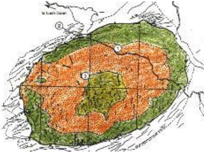
Fig. 39. Petrological map of the Fleet pluton, showing the main zones (after Stephens, 1997; taken from Parslow, 1968). Fine-grained biotite-muscovite granite (yellow); coarse-grained biotite-muscovite granite (orange); coarse-grained biotite granite (green).
