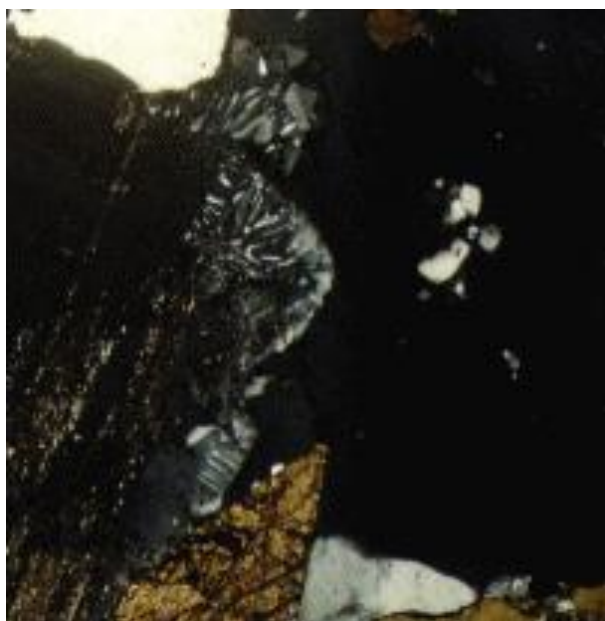
Fig. 7. Sericitized, albite-twinned plagioclase (left side) with myrmekite borders against K-feldspar (black, right side). Larger quartz crystals (white and cream), sphene (diamond, brown), and hornblende (brown, right corner). Loch Sunart granodiorite, porphyritic facies.
