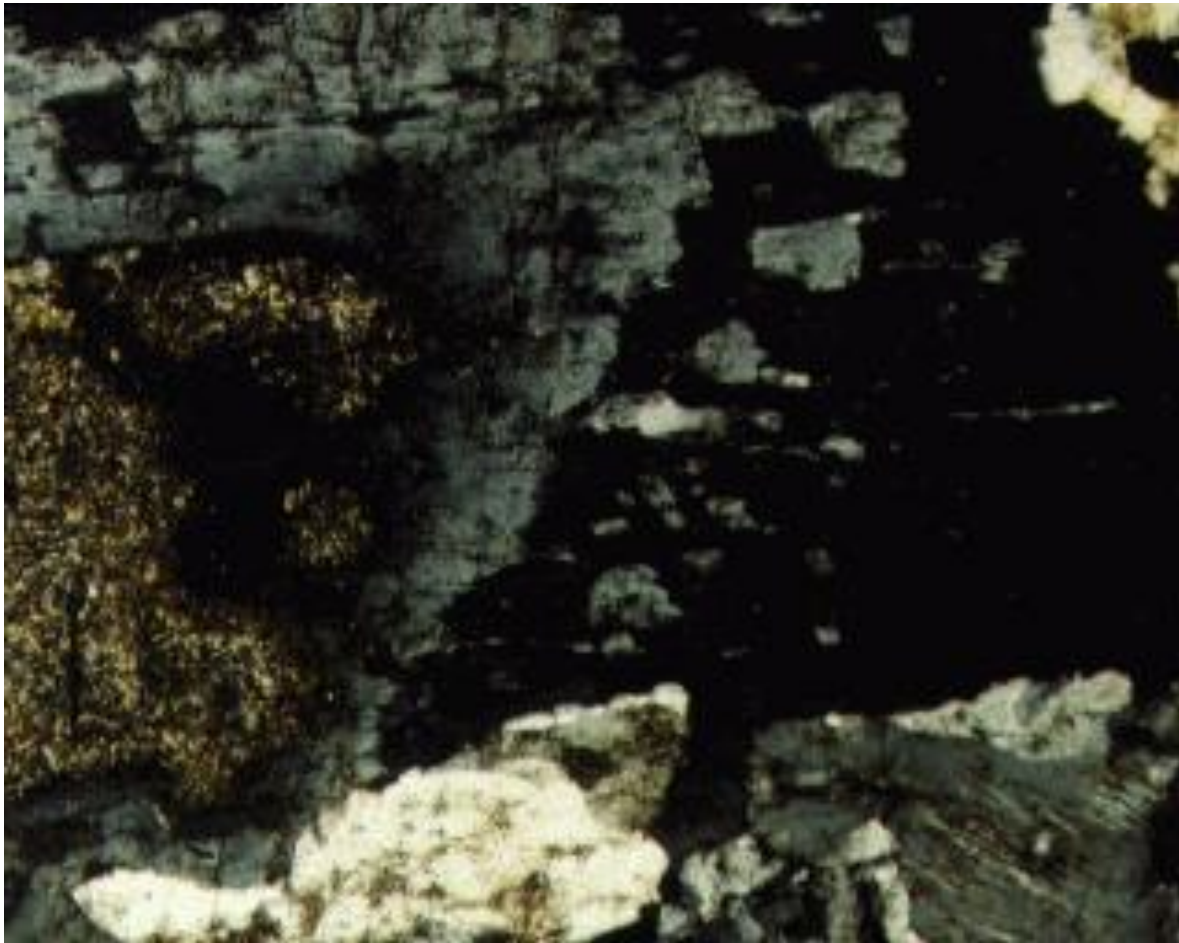
Fig. 18. Large zoned plagioclase (light gray) with sericitized central core (left side; brownish). Outer broad rim of the plagioclase is replaced by perthitic K-feldspar (black). Island remnants of the plagioclase in parallel optic continuity remain in the K-feldspar. Ratagain pluton.
