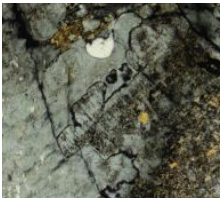
Fig. 38. Perthitic K-feldspar (left side; light gray) penetrating albite-twinned plagioclase (same light gray) along fractures (center). Island remnants of plagioclase (center) remain in the K-feldspar in parallel optical continuity. Biotite granite facies; Criffell pluton.
