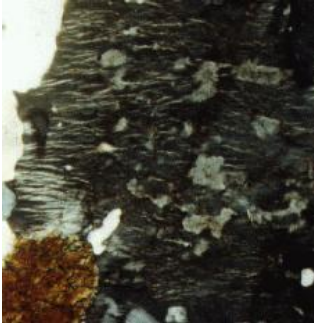
Fig. 20. Perthitic microcline (dark gray) with remnant irregular islands of plagioclase and plagioclase lamellae (light gray), both of which are optically continuous. Hornblende (brown). Quartz (white). Ratagain pluton.
