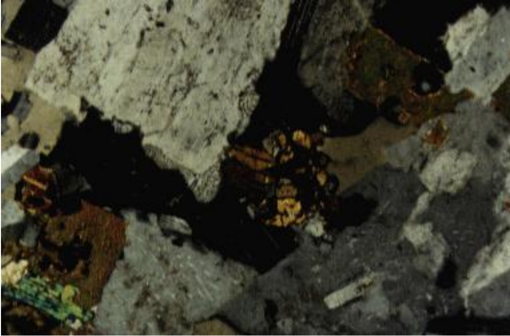
Fig. 43. Perthitic K-feldspar (black, light gray; center and bottom right) penetrating broken plagioclase crystals (lighter gray, top; and bottom right). Borders of plagioclase are myrmekitic (center). Biotite (brown, green). Pyroxene (brown, tan). In norite in the Doon pluton.
