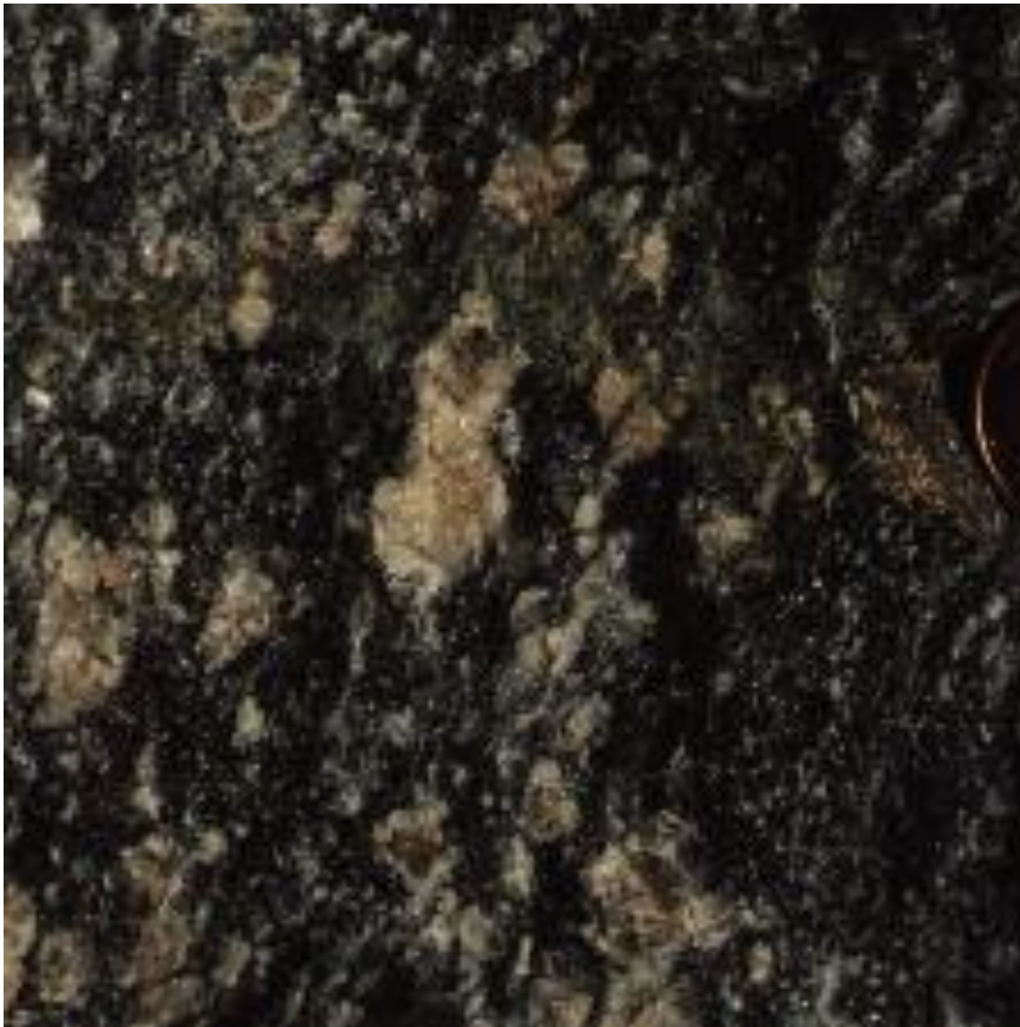
Fig. 16. Close-up photograph of Fig. 15, showing white rims on some of the pink-K-feldspar crystals.
