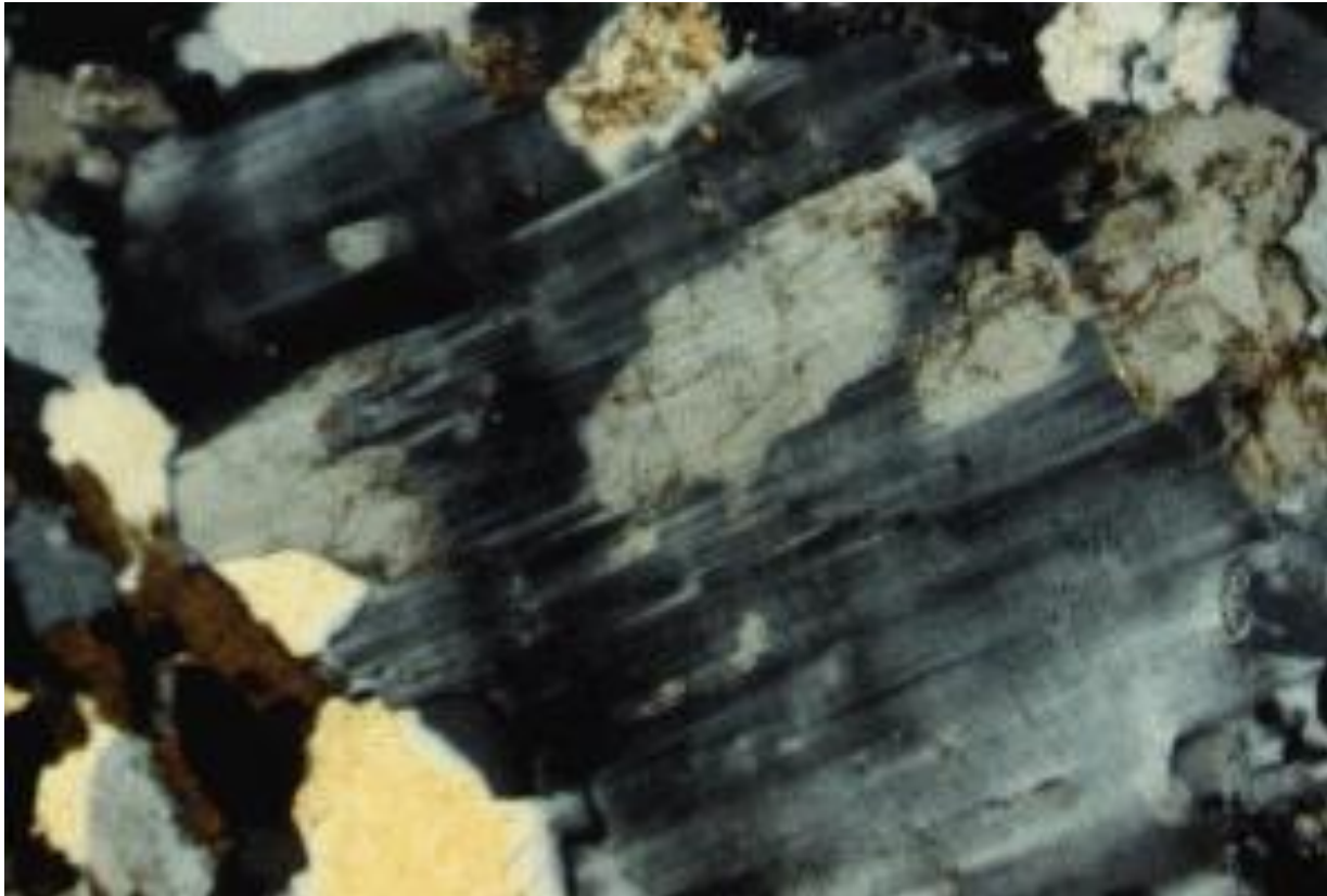
Fig. 18. Photomicrograph of K-feldspar (gray and black, cross-hatch twinned) with remnants of plagioclase (tan) which extend through the K-feldspar in parallel optical continuity. Ground mass minerals consist of quartz (cream, gray, white), biotite (brown), hornblende (brown), and additional plagioclase (tan, gray). In hand specimen, this K-feldspar would appear as a tiny pink crystal in the midst of the black plagioclase amphibolite.
