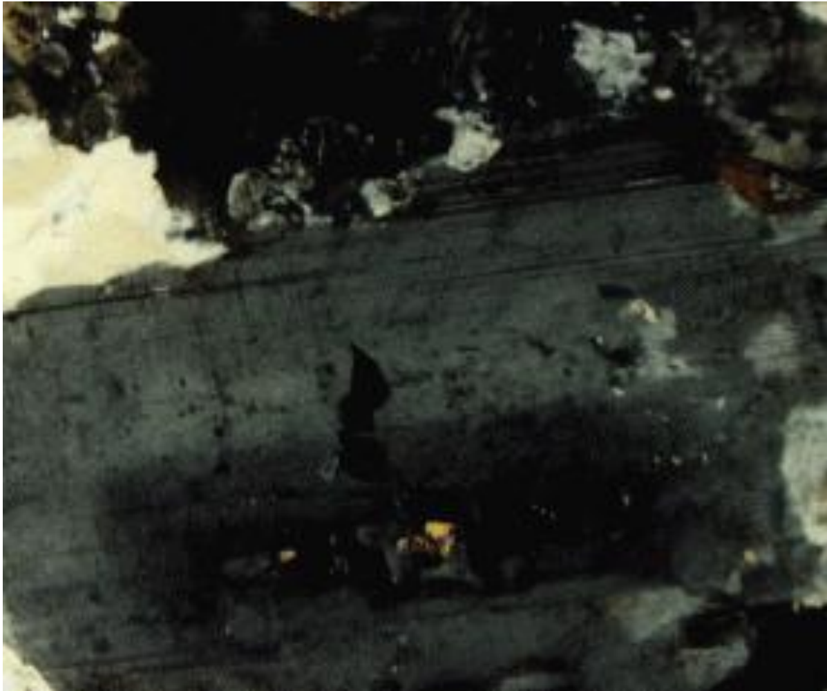
Fig. 22. Photomicrograph of myrmekite projecting into K-feldspar (black, top) and optically continuous with zoned non-quartz-bearing plagioclase (shades of gray, bottom) in granodiorite associated with the Marlboro plagioclase amphibolite.
