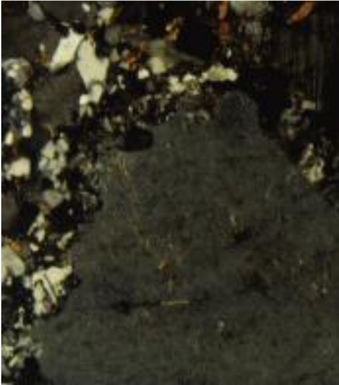
Fig. 26. Photomicrograph of aggregate myrmekite grains bordering K-feldspar (gray) at outcrop THREE. Ground mass consists of quartz, plagioclase, biotite, and hornblende of adjacent plagioclase amphibolite.
