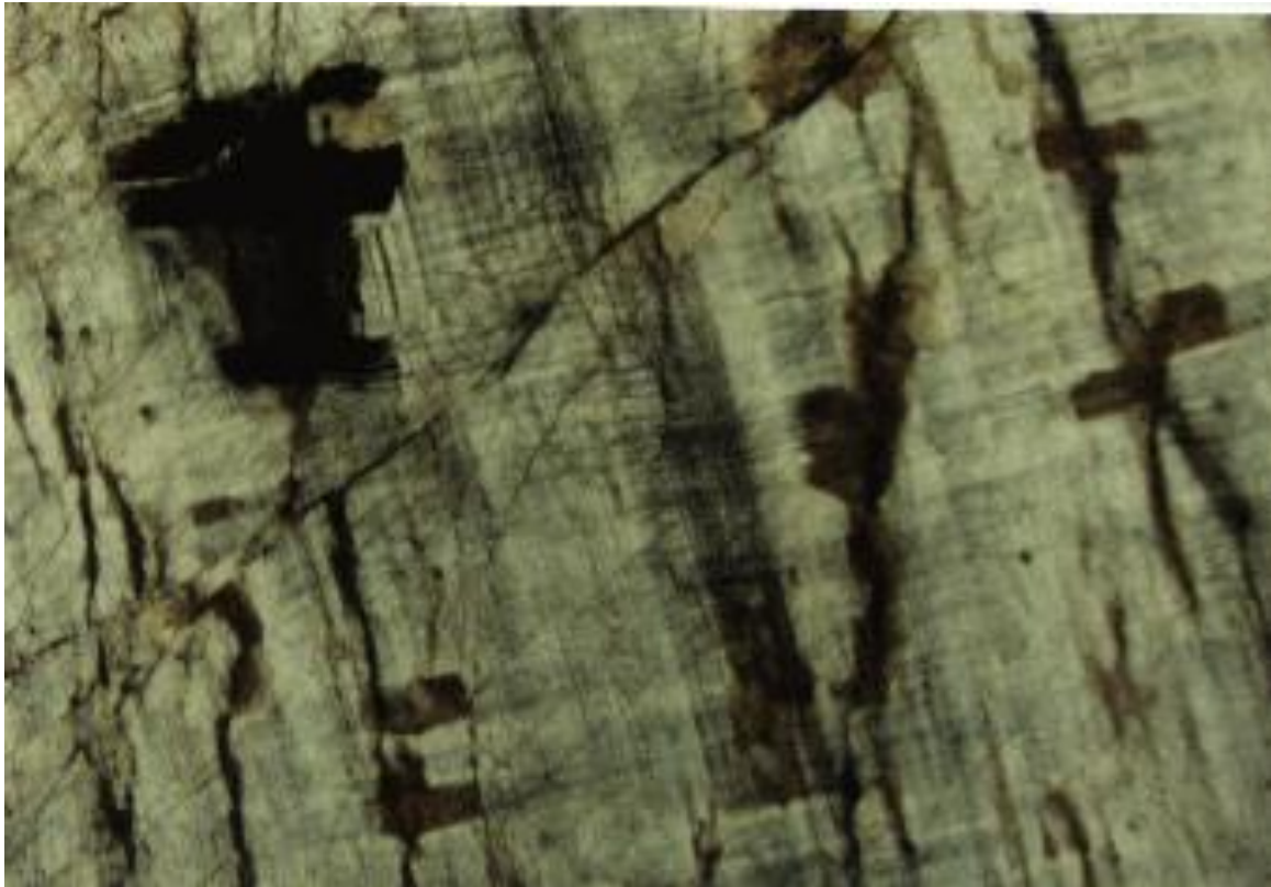
Fig. 23. Photomicrograph of K-feldspar (shades of gray, cross-hatch twinning), enclosing bent and broken, albite-twinned, plagioclase islands which are in optical continuity (tan, rectangular, and black and gray).
