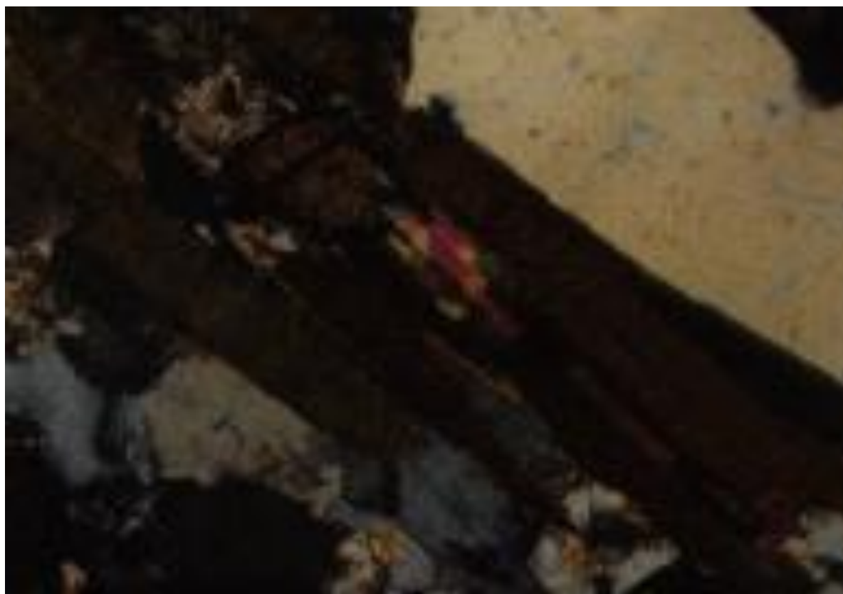
Fig. 3. Early stage of replacement of biotite by muscovite in relatively undeformed biotite granite.
