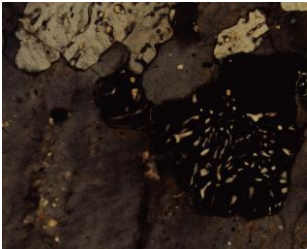
Fig. 4. Inclusions of wartlike myrmekite (black with white quartz vermicules; light gray with dark quartz vermicules) in the K-feldspar (gray).
