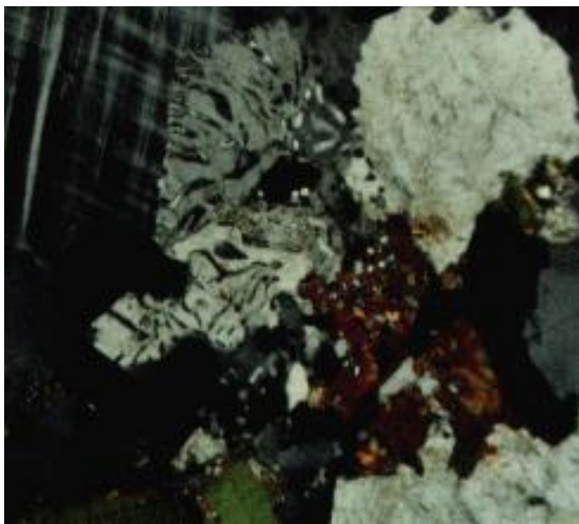
Fig. 6. Relatively coarse vermicules in myrmekite in the Thorr granodiorite west of southwest end of the Main Donegal granite. Epidote (reddish brown, center) with tiny quartz inclusions and biotite (green and brown) are coexisting minerals. K-feldspar (black and gray, cross-hatched twinning) is in upper left. Plagioclase (white, upper right) is adjacent to myrmekite.
