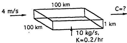
Input rate = Output rate + KCV
