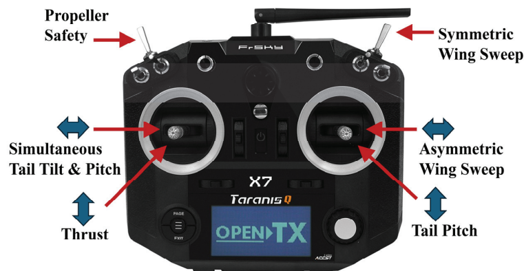
Figure 12. CGull's remote control mapping.
