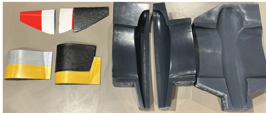
Figure 14. 3D-printed molds used for composite manufacturing.
