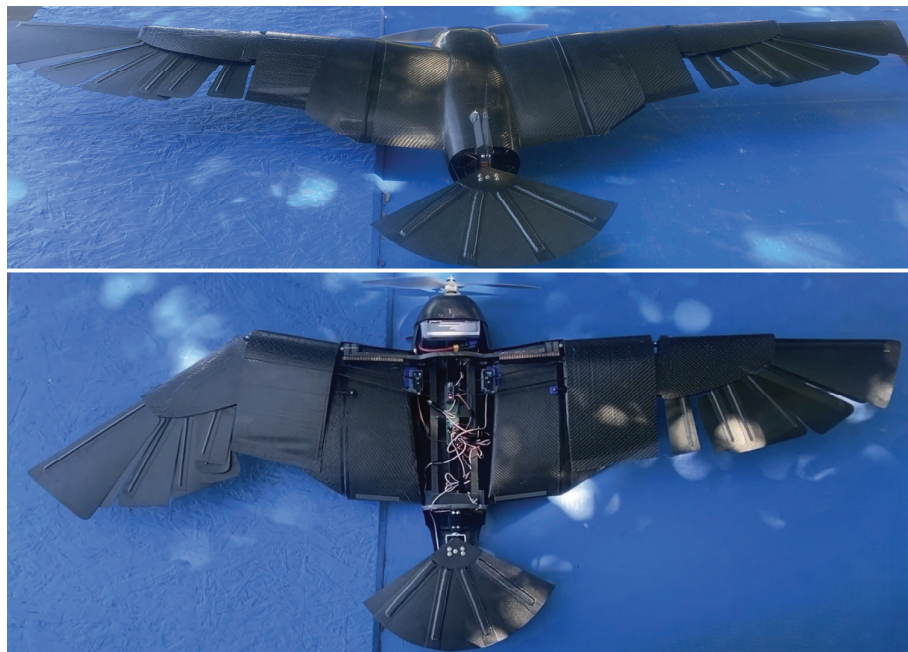
Figure 18. CGull prototype before the flight test (the top fuselage cover is removed, and the left wing is swept back in the bottom figure).
