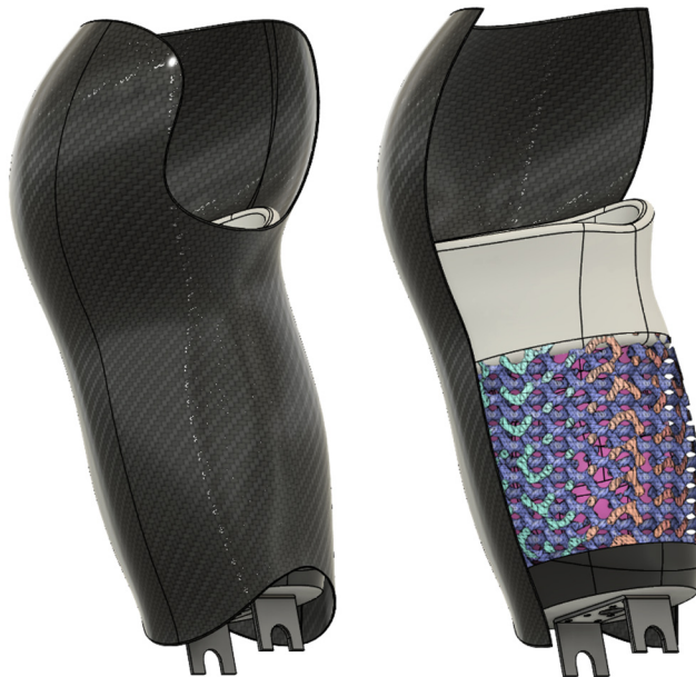
Figure 6: Side by side comparison of the bicep assembly which houses the multi-material arm socket, and 150 kg servo attachment.
