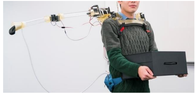
Fig. 1. The first prototype of the wearable robot arm; the human is carrying a box in both hands with the prototype of a wearable robot arm.
