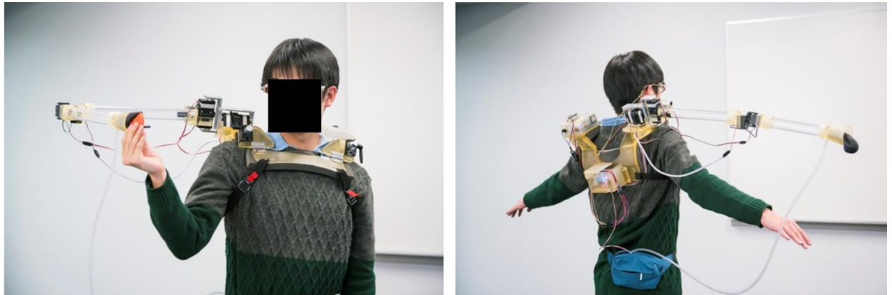
Fig. 2. The first prototype of the wearable robot arm; an articulated robot arm is attached to the shoulder position of the human [17]
