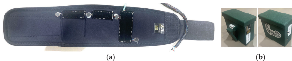
Figure 14. (a) Manufactured sensory feedback armband, (b) electronics box.
