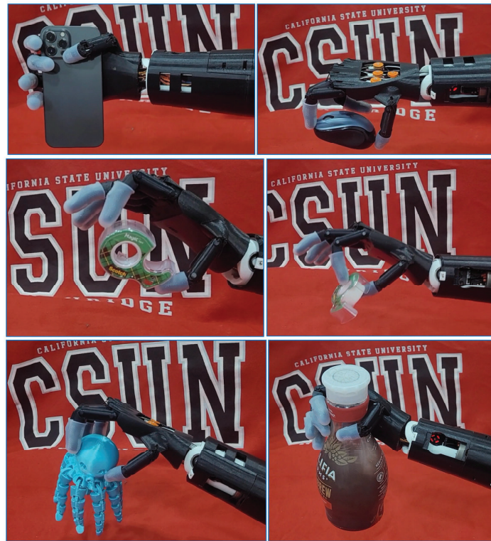
Figure 21. Infinity arm grips different objects using different grip patterns.
