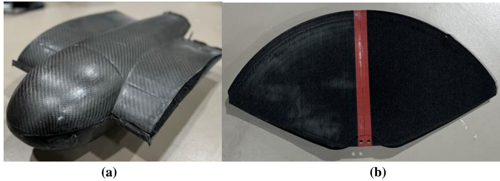
Fig. 15. (a) Composite structures: fuselage, (b) 3D-Printed PLA Aero Tail Structure
