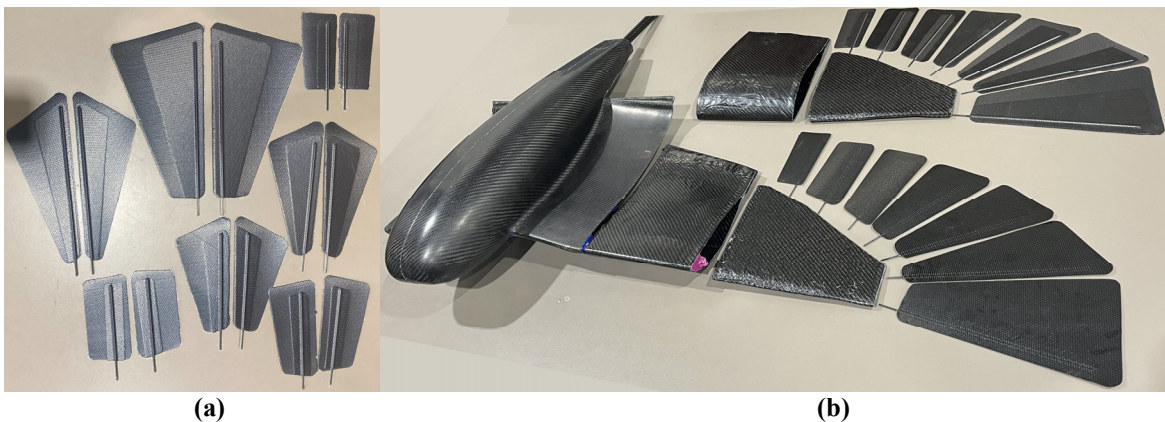
Fig. 12 (a) Wing composite feathers, (b) Composite structures: Fuselage and inner wing, middle wings, outer wings with feathers.
