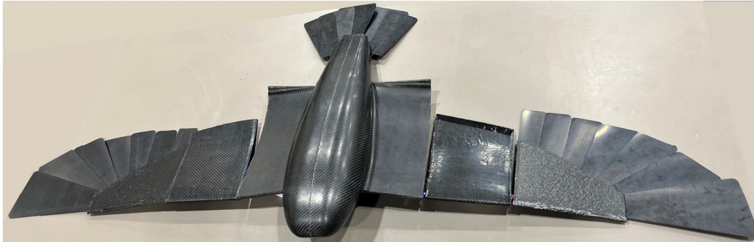
Fig. 15 Bottom view of CGull's prototype
