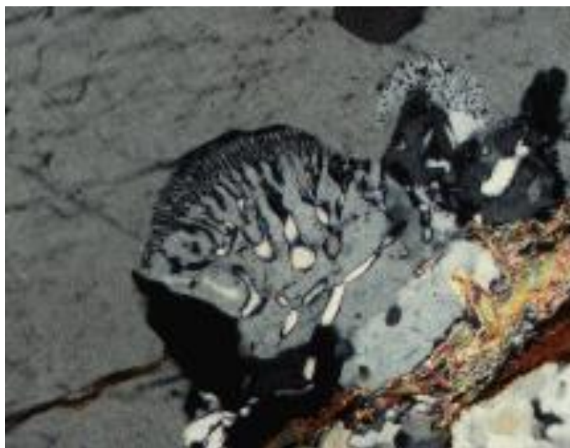
Fig. 5. Myrmekite (center, with branched vermicules) bordering K-feldspar megacrysts (gray, upper left). Quartz is light gray and white. Biotite is brown.
