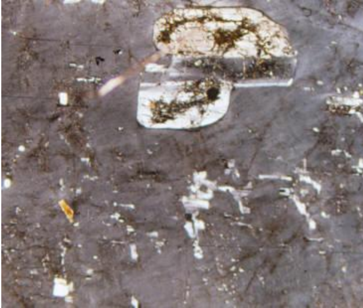
Fig. 13. Remnant islands of plagioclase (white; lower right) in parallel optical continuity occur in microcline (gray) below and altered, large, remnant island of albite-twinned plagioclase with rounded scalloped edges. Biotite (brown).
