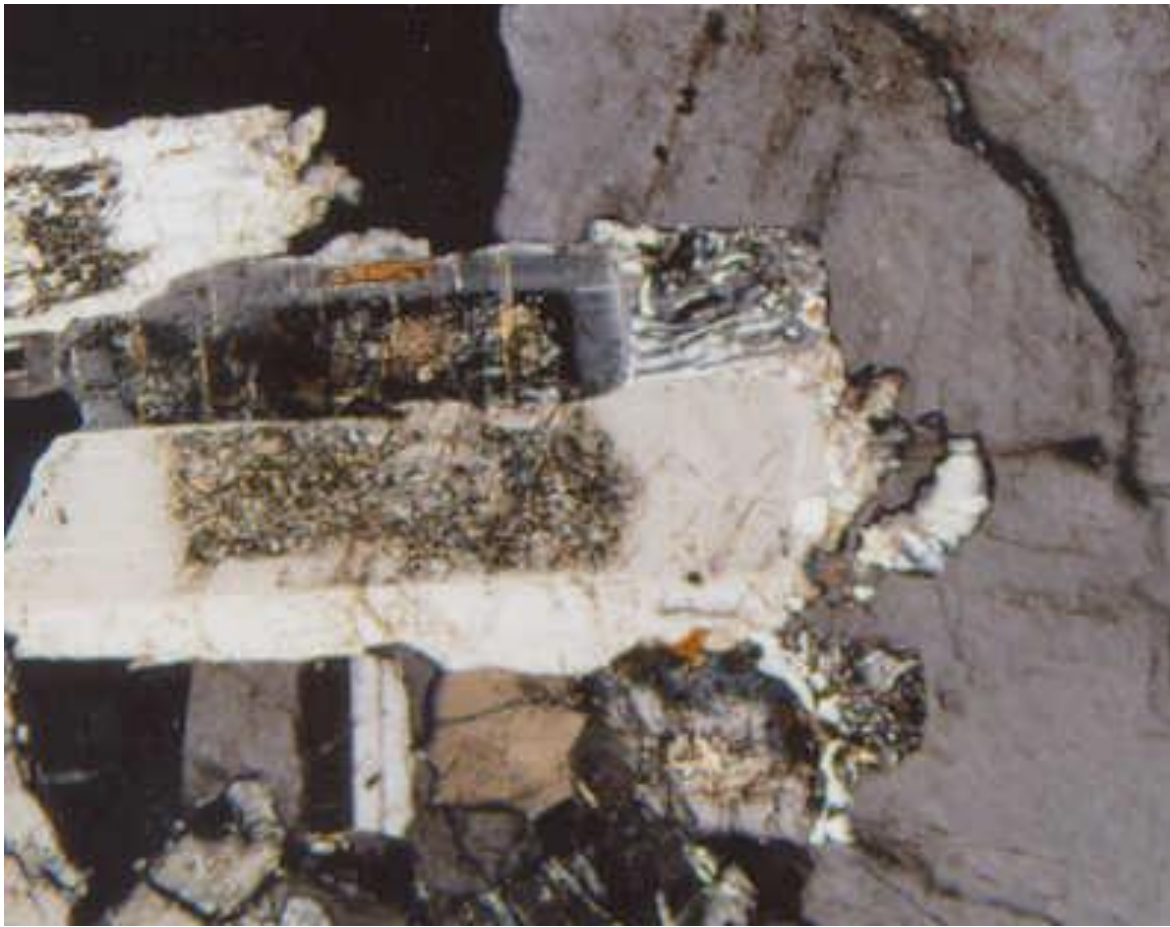
Fig. 18. Carlsbad-twinned and zoned plagioclase crystal with speckled, sericite-altered core. Remnant end of the plagioclase crystal (center; right) occurs as an island in microcline (gray; right side) and is in optical parallel alignment with larger plagioclase crystal (left side). Myrmekite with tiny quartz vermicules occurs on corners of plagioclase projecting into microcline.
