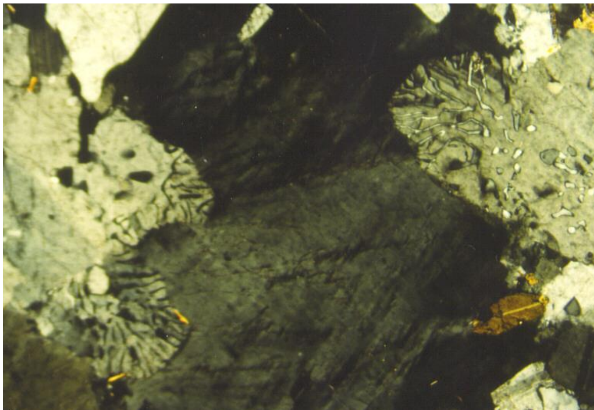
Fig. 7. Microcline (center; black, gray) penetrates and replaces non-quartz-bearing part of plagioclase next to the myrmekite (upper left quadrant; light gray and cream) along fractures (upper part of myrmekite; left side). Myrmekite also occurs on right side. Biotite (brown, light tan).
