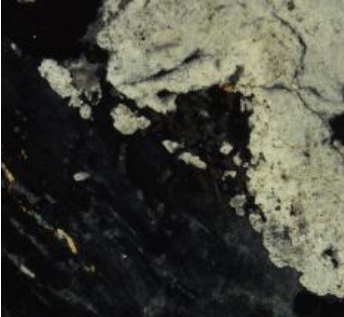
Fig. 22. Plagioclase (white). Microcline (black to dark gray). Microcline penetrates and replaces the plagioclase, leaving tiny island remnants of the plagioclase in optical parallel continuity.
