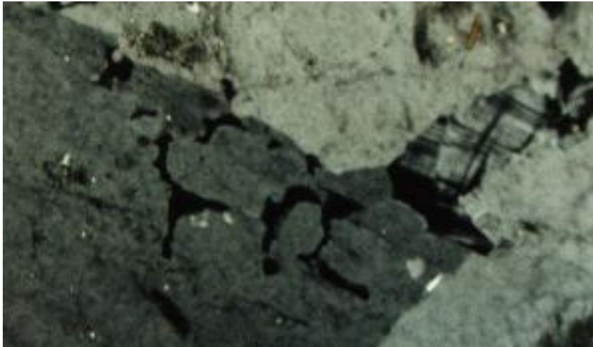
Fig. 3. Replacement of albite-twinned plagioclase (gray and light-gray) by irregular islands of K-feldspar (black and cross-hatched pattern) along microfractures.
