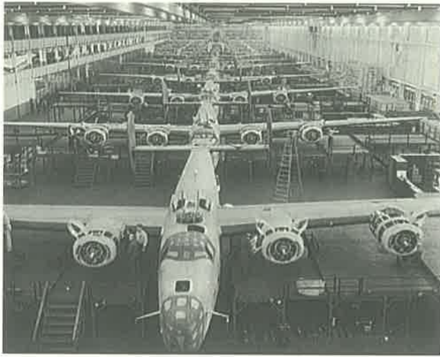
26 B-24 Liberators under construction. Henry Ford, the car manufacturer, set out to build a bomber every hour in his new factory near Detroit. Using mass-production methods, he achieved his aim by 1944.
