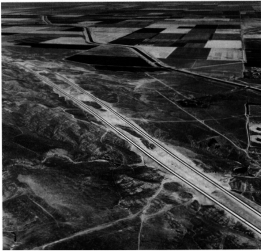
Figure 4. Figure 4. The familiar checkerboard pattern of the Township & Range land division system is especially pronounced in flat areas such as the San Joaquin Valley near Kettleman City. Photograph provided by the California Department of Transportation.
