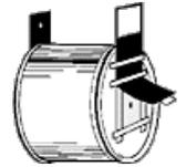
Pinhole camera made from a can.
