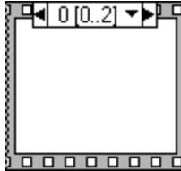
To take advantage of the inherent parallelism in LabVIEW, avoid overusing sequence structures. Sequence structures guarantee the order of execution and prohibit parallel operations. For example, asynchronous tasks that use I/O devices, such as PXI, GPIB, serial ports, and DAQ devices, can run concurrently with other operations if sequence structures do not prevent them from doing so.
