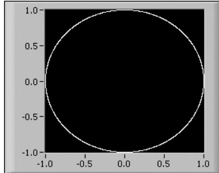
The XY graph can display plots containing any number of points. The XY graph also accepts several data types, which minimizes the extent to which you must manipulate data before you display it.
