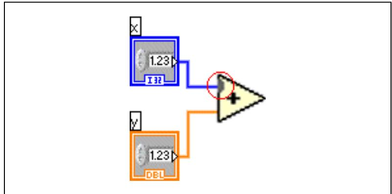
Coercion dots can cause a VI to use more memory and increase its run time. Try to keep data types consistent in the VIs you create.
