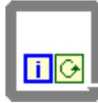
The While Loop executes the subdiagram until the conditional terminal, an input terminal, receives a specific Boolean value. The default behavior and appearance of the conditional terminal is **Stop if True**, shown as follows.
