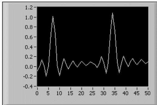
The waveform graph can display plots containing any number of points. The graph also accepts several data types, which minimizes the extent to which you must manipulate data before you display it.
