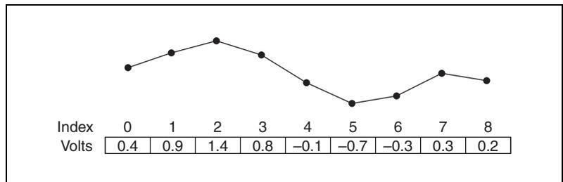
A more complex example of an array is a graph represented as an array of points where each point is a cluster containing a pair of numeric values that represent the X and Y coordinates, as shown in the following figure.
