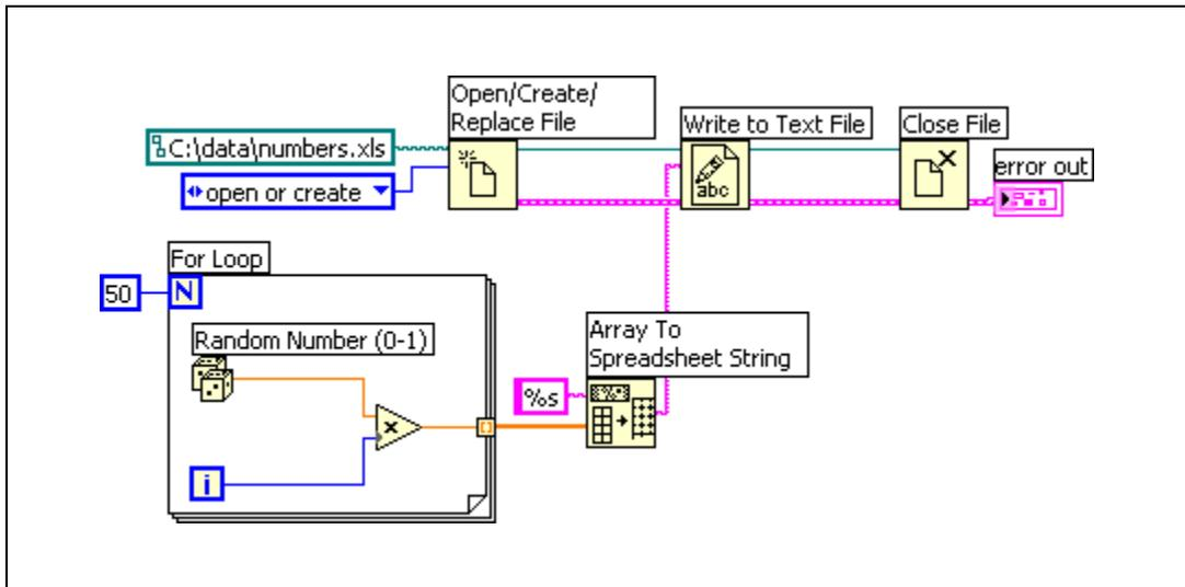
Compare the previous block diagram to the Write to Spreadsheet VI, which completes the same task. The previous block diagram uses individual functions for each file operation, including using the Array To Spreadsheet String function to format the array of numbers as a string. The Write To Spreadsheet File VI completes multiple file operations, including opening the file, converting the array of numbers to a string, and closing the file.
