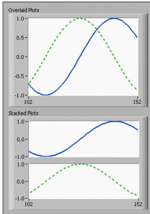
Right-click the chart and select **Stack Plots** from the shortcut menu to view the chart plots as multiple vertical scales. Right-click the chart and select **Overlay Plots** to view the chart plots as a single vertical scale.
