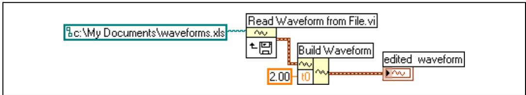
The Read Waveform from File VI also reads multiple waveforms from a file. The VI returns an array of waveform data, which you can display in a multiplot graph. If you want to access a single waveform from a file, you must index the array of waveform data, as shown in the following block diagram. The VI accesses a file that includes multiple waveforms. The Index Array function reads the first and third waveforms in the file and plots them on two separate waveform graphs.
