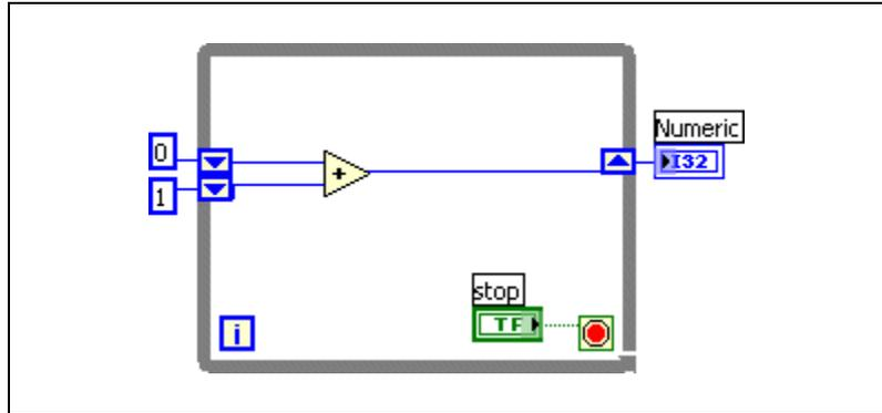
If you add another element to the left terminal in the previous figure, values from the last two iterations carry over to the next iteration, with the most recent iteration value stored in the top shift register. The bottom terminal stores the data passed to it from the previous iteration.
