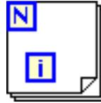
The value in the count terminal (an input terminal), shown as follows, indicates how many times to repeat the subdiagram.
