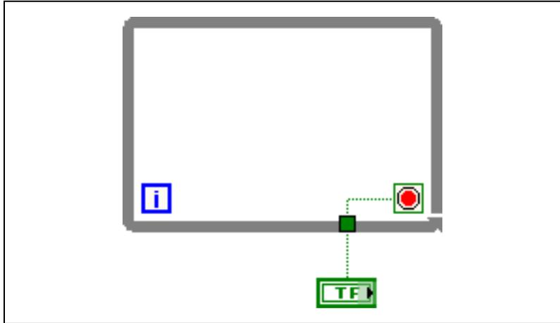
Changing the value of the control does not stop the infinite loop because the value is only read once, before the loop starts. To stop an infinite loop, you must abort the VI by clicking the **Abort Execution** button on the toolbar.
