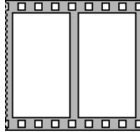
The Stacked Sequence structure, shown as follows, stacks each frame so you see only one frame at a time and executes frame 0, then frame 1, and so on until the last frame executes.
