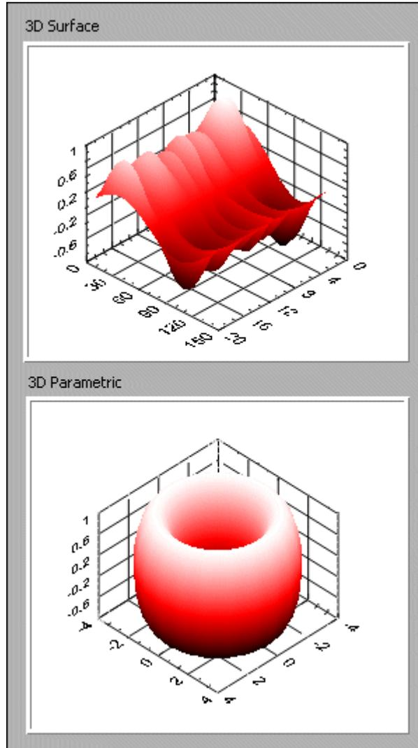
The 3D graphs use ActiveX technology and VIs that handle 3D representation. When you select a 3D graph, LabVIEW places an ActiveX container on the front panel that contains a 3D graph control. LabVIEW also places a reference to the 3D graph control on the block diagram. LabVIEW wires this reference to one of the three 3D Graph VIs.
