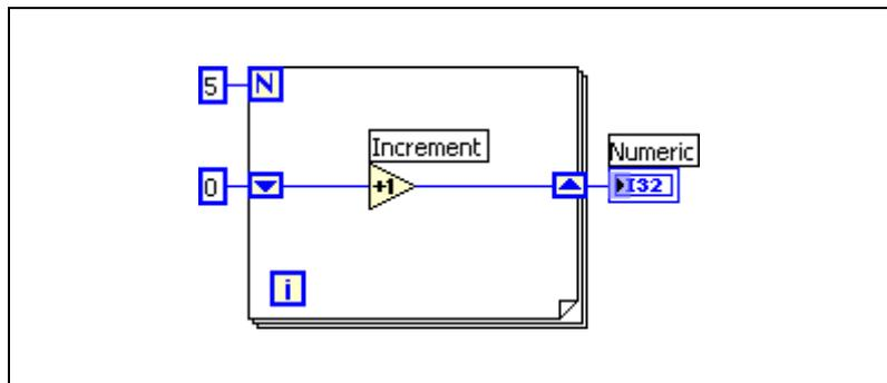
In the previous figure, the For Loop executes five times, incrementing the value the shift register carries by one each time. After five iterations of the For Loop, the shift register passes the final value, 5, to the indicator and the VI quits. Each time you run the VI, the shift register begins with a value of 0.
