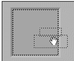
To create a cluster constant on the block diagram, select a cluster constant on the **Functions** palette, place the cluster shell on the block diagram, and place a string constant, numeric constant, or cluster constant in the cluster shell. You can use a cluster constant to store constant data or as a basis for comparison with another cluster.
