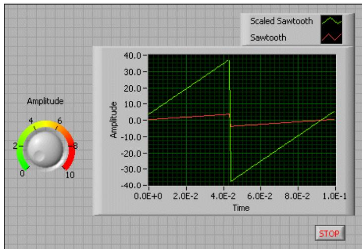
You build the front panel using controls and indicators, which are the interactive input and output terminals of the VI, respectively. Controls are knobs, push buttons, dials, and other input mechanisms. Indicators are graphs, LEDs, and other output displays. Controls simulate instrument input mechanisms and supply data to the block diagram of the VI. Indicators simulate instrument output mechanisms and display data the block diagram acquires or generates.
