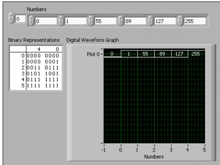
Right-click the y-scale and select **Expand Digital Buses** from the shortcut menu to plot each sample of digital data. Each plot represents a different bit in the digital pattern.
