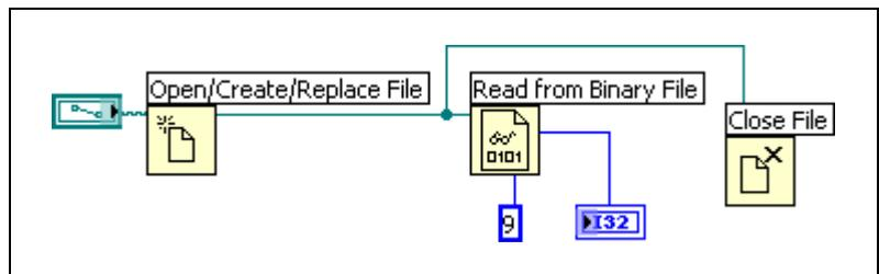
The following block diagram establishes a dependency by wiring an output of the Read from Binary File function to the Close File function. The Close File function does not run until it receives the output of the Read from Binary File function.
