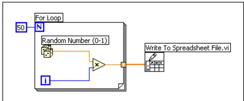
The open, read, and write functions expect a file path input. If you do not wire a file path, a dialog box appears for you to specify a file to read from or write to.
