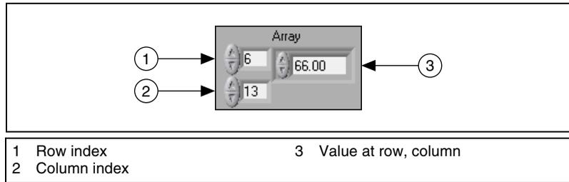
Rows and columns are zero-based, meaning the first column is column 0, the second column is column 1, and so on. Changing the index display for the following array to row 1, column 2 displays a value of **6**.
