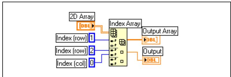
To access multiple consecutive values in an array, expand the Index Array function, but do not wire values to the index inputs in each increment. For example, to retrieve the first, second, and third rows from a 2D array, expand the Index Array function by three increments and wire 1D array indicators to each sub-array output.
