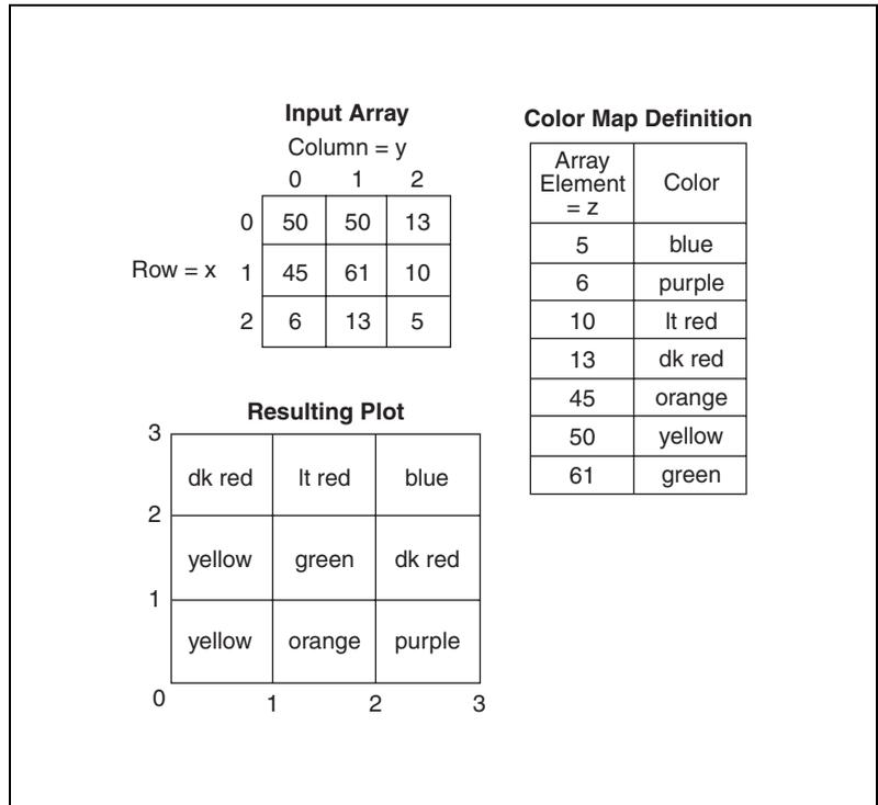
The rows of the data pass into the display as new columns on the graph or chart. If you want rows to appear as rows on the display, wire a 2D array data type to the graph or chart, right-click the graph or chart, and select **Transpose Array** from the shortcut menu.
