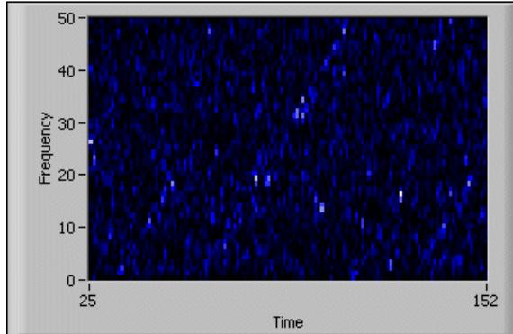
The intensity chart shares many of the optional parts of the waveform chart, including the scale legend and graph palette, which you can show or hide by right-clicking the chart and selecting **Visible Items** from the shortcut menu. In addition, because the intensity chart includes color as a third dimension, a scale similar to a color ramp control defines the range and mappings of values to colors.
