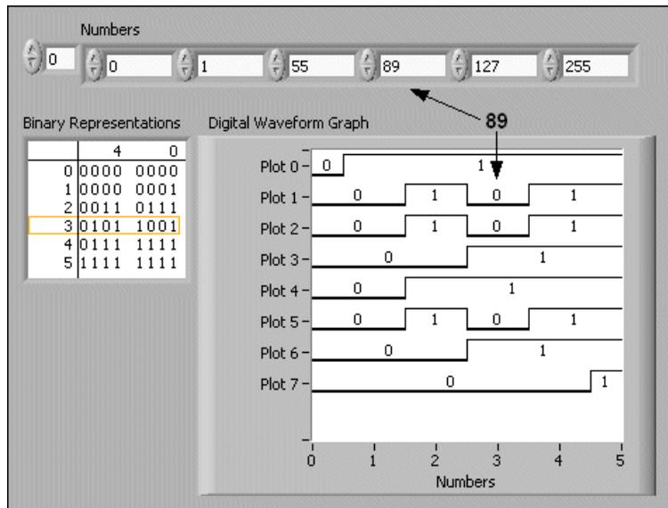
The **Binary Representations** digital indicator displays the binary representations of the numbers. Each column in the table represents a bit. For example, the number 89 requires 7 bits of memory (the 0 in column 7 indicates an unused bit). Point 3 on the digital waveform graph plots the 7 bits necessary to represent the number 89 and a value of 0 to represent the unused eighth bit on plot 7.
