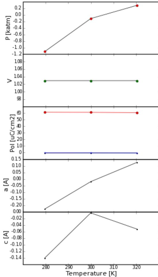
Figure 1: Pressure, Volume, Polarization verse temperature for MD simulation of LiNbO<sub>3</sub> (T300 -c ).
