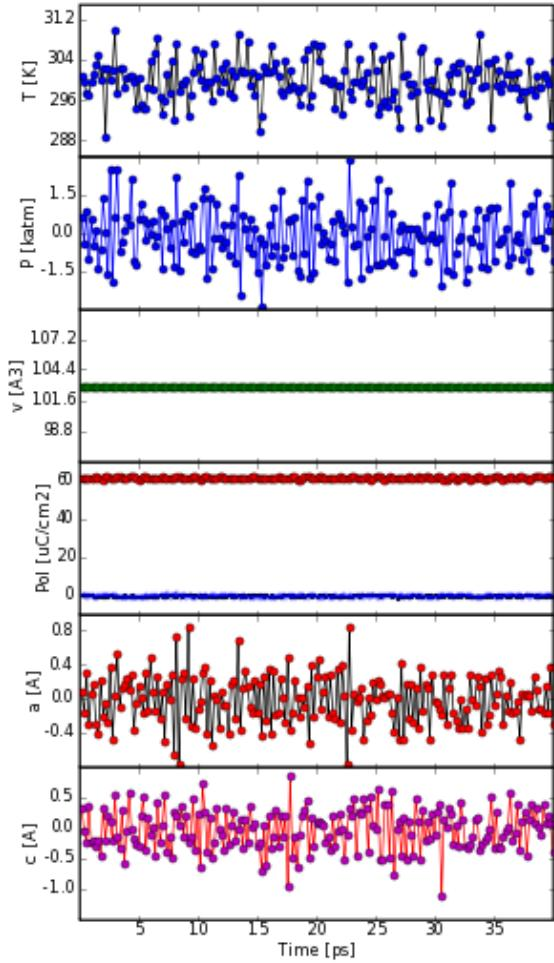
Figure 3: Temperature, Pressure, Volume, Polarization verse time for MD simulation of LiNbO<sub>3</sub> at target temperature T=300 K (T300).
