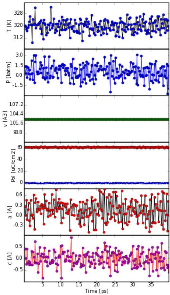
Figure 4: Temperature, Pressure, Volume, Polarization verse time for MD simulation of LiNbO<sub>3</sub> at target temperature T=320 K (T300).
