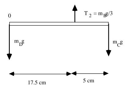
We have used the 3rd law to write  $T_2 = m_B g/3$  as the tension on the top string.
