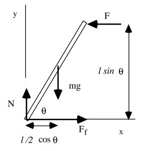
force of the floor on the ladder from the torque equation. There is no vertical component of force on the ladder due to the wall since the wall is frictionless. Equilibrium requires
