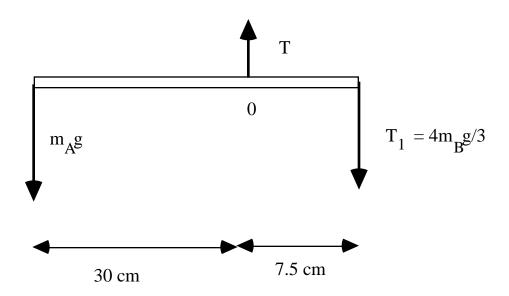
We have used the 3rd law to write  $T_1 = 4m_Bg/3$  as the tension on the string to the right.
