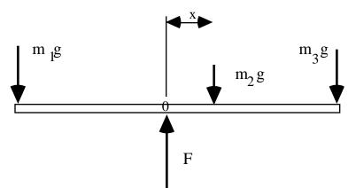
from the fulcrum. Placing the origin at the fulcrum eliminates the force due to the fulcrum from the torque equation
