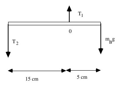
Taking the origin as shown, eliminates  $T_1$  from the torque equation
