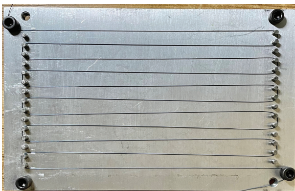
Fig. 1. SMA wire placement fixture used for manufacturing test laminates.
