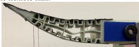
Fig. 17 Active rib morphing with 700 gm weight
