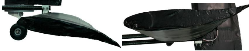
Fig. 20 Horizontal (left) and Vertical (right) stabilizers camber actuation
