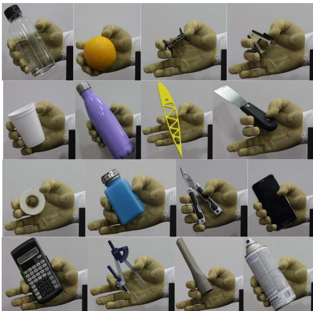
Figure 17. MataPro-1 gripping different objects.
