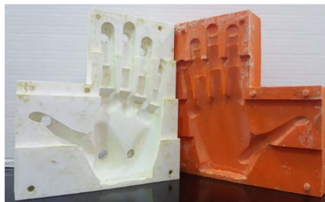
Figure 10. Two-piece mold for the whole hand.
