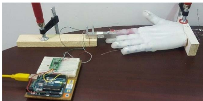
Figure 15. Experimental setup to measure fingertip force.
