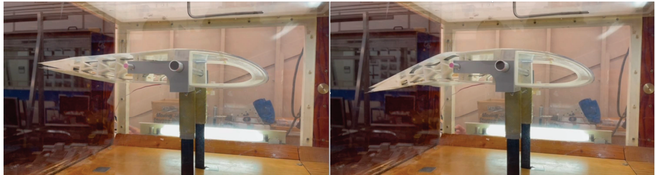
Figure 19. Two views for the assembled and camber-morphed tail stabilizer model.
