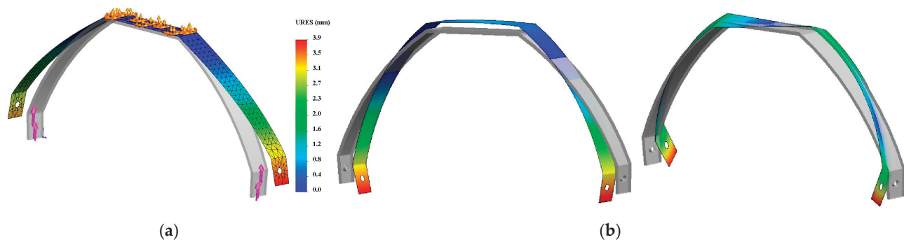
Figure 13. (a) Displacement of main landing gear in static study; (b) Main landing gear's 1st (left, 70 Hz) and 2nd (right, 170 Hz) NRB mode shapes.
