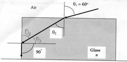
(a) (20 points) Find the value of n for which we have a total internal reflection on the vertical surface of the paperweight (Useful equations:  $\sin(90^{\circ} - \theta) = \cos\theta$
