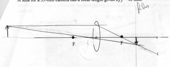
(8 pt) a) How close to the film should the lens be placed to form a sharp image of an object that is
