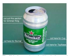
The Heineken can has raised bands that provide perfect diameter and spacing for all of the parts. Three cans are needed to make the stove. Another kind of pop or beer can actually works better for for the top/base. Cut with a knife and finish with large scissors.
