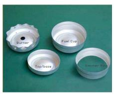
Top/base should be shorter than shown (about 1/2" tall). The Burner (3/4" t ll) is cut off just below the first band. The Fuel Cup is cut off at the top of the band (making it about 1 1/4" tall). The Simmer ring uses a top band and top flat section (about 1" tall).
