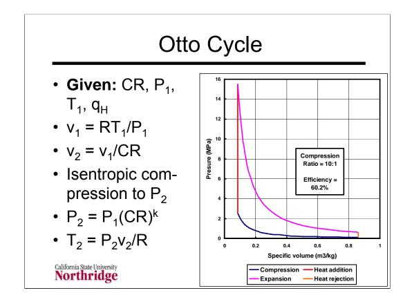
This chart shows the diagram of an Otto cycle, the idealization of the cycle in a gasoline engine. It also shows the start of the cycle analysis. The compression and expansion are assumed to be adiabatic. The only heat transfer in the cycle is the constant volume heat addition and rejection. The remainder of the analysis is shown below.
