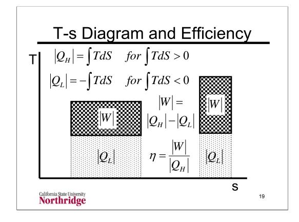
The temperature-entropy or T-s diagram is often used to plot cycles because it shows provides a visual way of comparing cycle efficiency, once you are familiar with the underlying relations.
