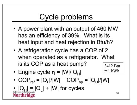
We can apply the efficiency equation to the work rate (power) and the heat input rate. This gives  $|Q_H| = |W| / \eta$ . = (460 MW)/ 39% = 1179 MW  $|Q_H| = (1179 \text{ MW})(1000 \text{ kW/MW})(3412 \text{ Btu/kWh}) = 4.025 \times 10^9 \text{ Btu/h}$  $|Q_L| = |Q_H| - |W| = 4.025 \times 10^9 \text{ Btu/h} - (460 \text{ MW}) (1000 \text{ kW/MW})(3412 \text{ Btu/kWh}) = 2.455 \times 10^9 \text{ Btu/h}$
