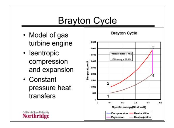
The Brayton cycle shown here uses the typical idealizations of the air standard cycle. Air is the working fluid. Combustion is modeled as a heat addition and the exhaust process is modeled as a heat rejection. The analysis of this cycle is similar to that of the Otto cycle, except that the heat additions take place at constant pressure so that  $q = \Delta h = c_p \Delta T$ .
