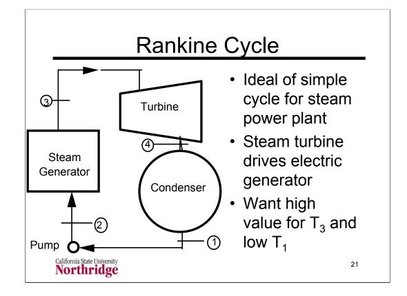
The application of the cycle idealizations to this simple Rankine cycle gives the following results. In this cycle heat is added in the steam generator and is rejected in the condenser. The net work output from the cycle is the difference between the work output from the turbine and the work input to the pump.
