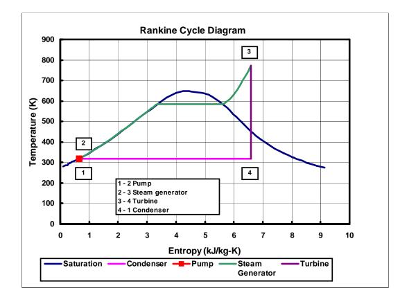
The state points for one particular example of a Rankine cycle (with a turbine inlet pressure and temperature of 10 MPa and 500°C and a condenser pressure of 10 kPa is shown on this diagram. The temperature increase in the pump is so small that the difference between the inlet and exit does not show on this diagram.
