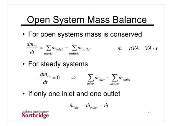
The equation relating mass flow rate, density (or specific volume), velocity, and cross sectional area is a fundamental relation among these variables. This is sometimes called the continuity equation. It applies to both steady and unsteady systems.
