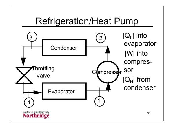
The simple refrigeration cycle shown here is characterized by an evaporator pressure,  $P_{evap}$ , and a condenser pressure  $P_{cond}$  that is higher that the evaporator pressure. The compressor is assumed to be isentropic and the throttling valve adds no heat or work so the enthalpy change across the valve is zero.
