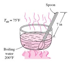
edge of the pot. The perimeter of the spoon is 2(0.08 in + 0.5 in) = 1.16 in = 0.09667 ft. If we use the equation for a finite length fin with an end correction for convection, we have  $L_c = L + A_c/p = 7 \text{ in} + (0.04 \text{ in}^2)/(1.16 \text{ in}) = 7.034 \text{ in}$ . The equation for the temperature profile along a fin is given below.
