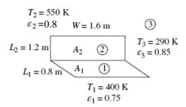
sides of the triangular enclosure (one flat surface that joins the outer edges of the horizontal and vertical surfaces shown and two triangular surfaces at the ends) are at 290 K and can be considered to have an emissivity of 0.85. Determine the net rate of radiation heat transfers between the two surfaces, and between the horizontal surface and the surroundings. (Problem and figure P13-45 from Çengel, Heat and Mass Transfer.)
