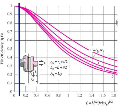
figure can be computed as follows:  $r_{2c} = r_2 + t/2 = 0.03 \text{ m} + (0.001 \text{ m})/2 = 0.0305 \text{ m}$ ;  $L_c = L + t/2 = 0.005 \text{ m} + (0.001 \text{ m})/2 = 0.0055 \text{ m}$ ;  $A_p = L_c t = (0.0055 \text{ m})(0.001 \text{ m}) = 5.5 \times 10^{-6} \text{ m}^2$ . We can now compute the parameters required to find the efficiency in Figure 3-43.
