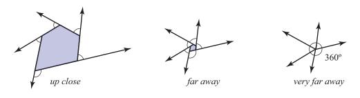
**Base Point Method.** Fix a point *P* and draw segments at *P* parallel to the sides of the polygon as shown. This creates angles congruent to the exterior angles of the polygon whose sum is  $360^{\circ}$ .
