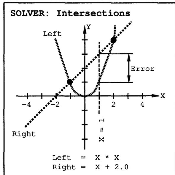
The user specifies a range of values and the program simply tries many random values within the range and evaluates the two equations storing the minimum distance between the two equations.
