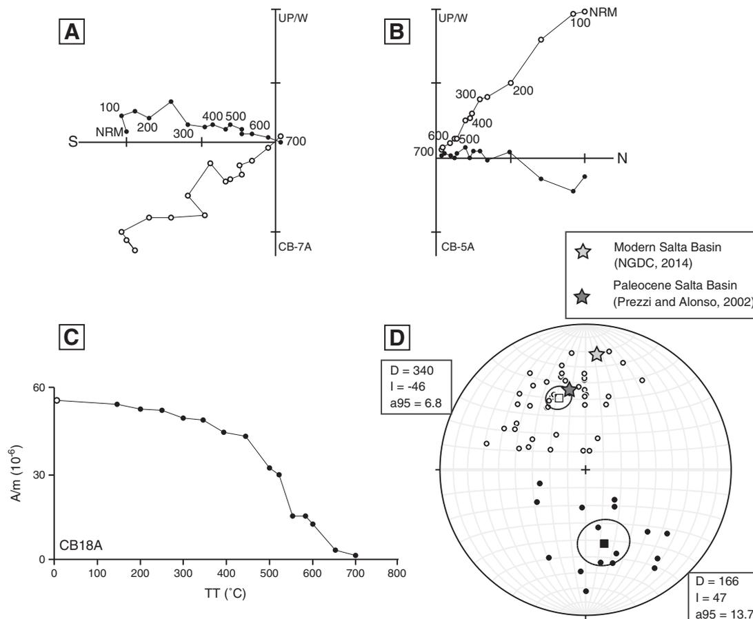
**Fig. 2.** Magnetostratigraphic results including: example vector endpoint diagrams for normal (A) and reversed (B) samples with thermal demagnetization steps; example thermal decay diagram for a fully demagnetized sample (C); and (D) a stereoplot of characteristic remanent magnetizations (ChRM) for all samples with Fisher mean values (squares), a95 circles, and modern and Paleocene poles for NW Argentina.
