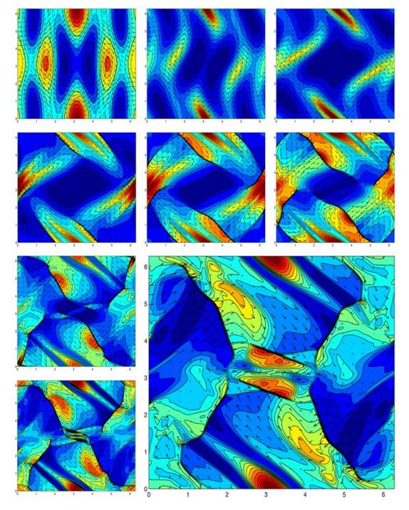
Fig. 1. Evolution of density with superimposed xz-velocity field, from left to right and top to bottom: density contours from t = 0.003: top-left corner to t = 2.7: lower left corner, displayed at (approximately) 0.375 time intervals. Large image in the lower right corner displays the solution at t = 3, density ranges from 1.2 to 6.1, and the maximum value of ||v|| is 1.7. There are 16 contour lines: red—high value; blue—low value.
