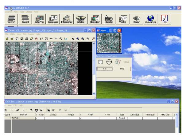
A new Viewer has appeared (Viewer #2). This contains a close-up of the areas in Viewer #1 which is enclosed by the white ("linked") box. In addition a "Geo Correction Tools" window has appeared at the top of the screen, and a "GCP Tool" at the bottom:
