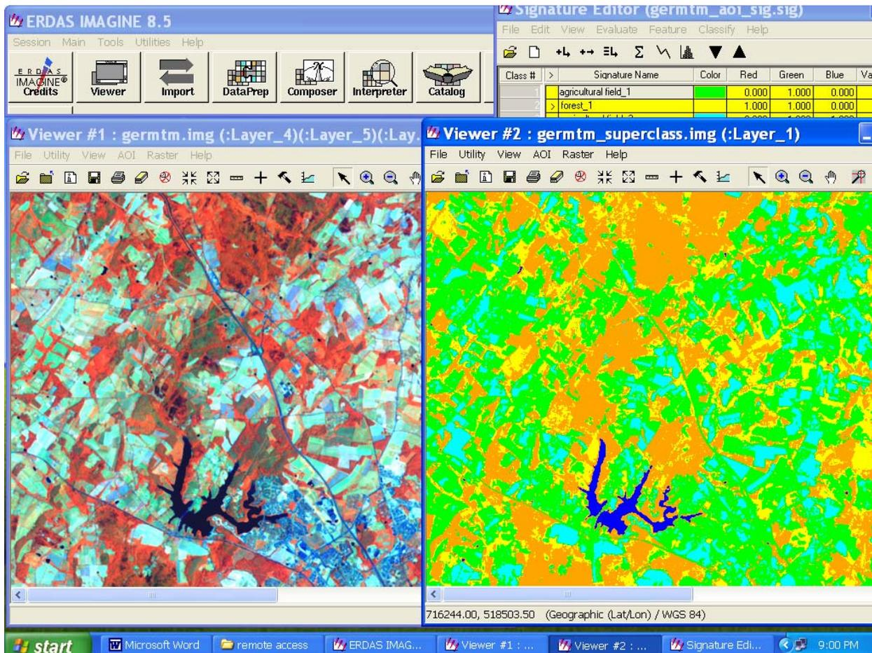
The original image is on the left. The classified one on the right. Now classify your image using a different rule (e.g. minimum distance), and save it under another name (e.g. <yourfile\_class2.img>).
