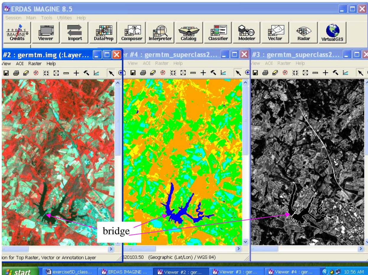
In the images above the left panel shows the unclassified image, the middle panel shows a classification done using minimum distance, and the right panel shows the distance file for this classification. You can see that the computer had some trouble
