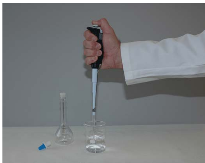
Figure 6.6 Liquid being drawn into the tip of a mechanical pipet
