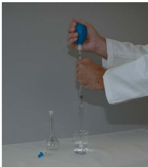
Figure 6.5 Liquid being drawn into a transfer pipet. It is calibrated to deliver a fixed volume.
