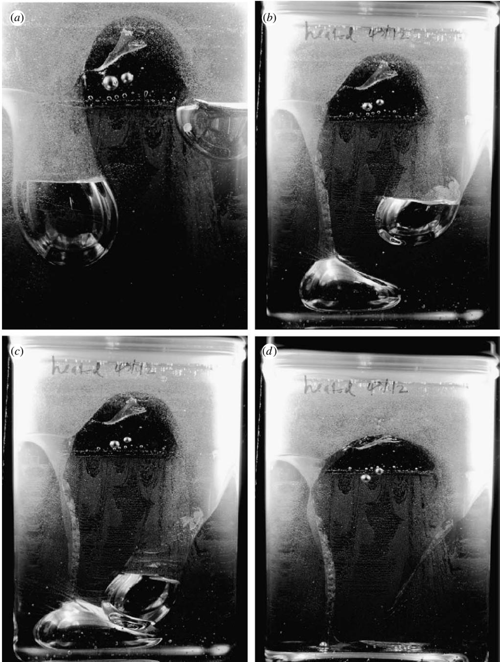
Figure 6. (*a–d*) Time sequence showing the development of half-diapirs and trailing conduits following Rayleigh–Taylor instability of a liquid gallium layer between two less dense but more viscous sucrose solution layers. Gallium diapir diameter on (*a, c*) is 4.5 cm. Total descent time from (*a*) to (*d*) is 10 min.
