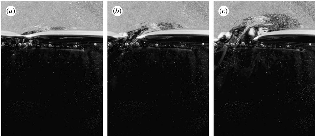
Figure 5. (a–c) Time sequence showing gallium layer segmentation during Rayleigh–Taylor instability of the three-layer fluid system in figure 4.
