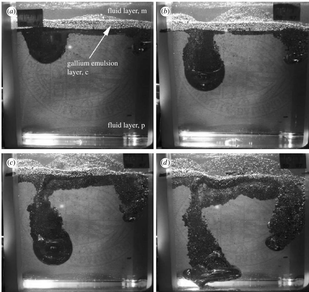
Figure 8. (*a, b*) Time sequence showing the development of Rayleigh–Taylor instability of an initial gallium emulsion layer between two less dense but more viscous sucrose solution layers. (*c, d*) The growth of a gallium emulsion plume; the upper/lower density and viscosity ratios are 0.9 and 0.01, respectively, and the initial emulsion layer thickness is 1.0 cm. Scale is visible near the upper fluid layer. Total experiment time from (*a*) to (*d*) is 52 min.
