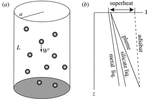
Figure 9. (a) Sketch of a steady-state metal–silicate mantle plume conduit used in the analysis, showing liquid metal drops sinking through a silicate magma matrix. (b) Schematic distribution of temperature along the plume, including metal and silicate melting lines, metal adiabat, plume temperature profile and core superheat.
