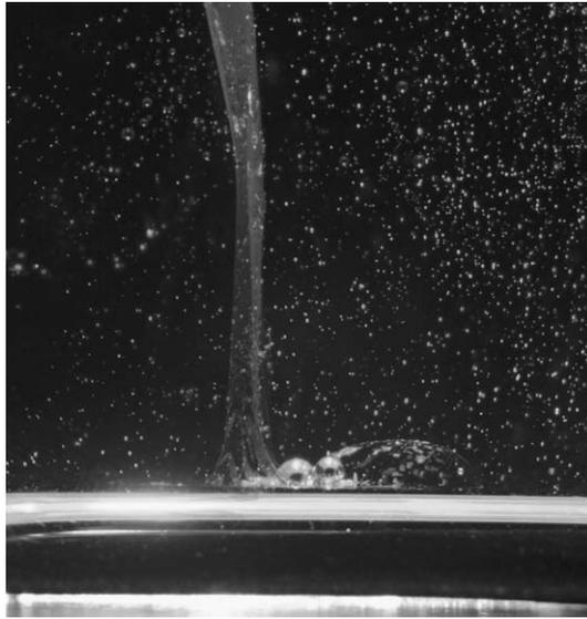
Figure 7. Structure of a positively buoyant thermochemical plume evolved from the trailing conduit of a negatively buoyant gallium plume.
