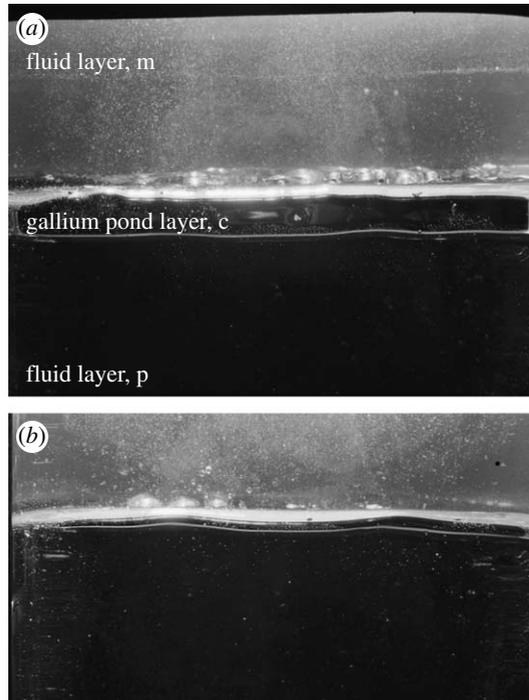
Figure 4. (a) Onset of Rayleigh–Taylor instability of a liquid gallium layer between two less dense but more viscous sucrose solution layers. The upper/lower density and viscosity ratios are 0.9 and 0.01, respectively, and the gallium layer thickness is initially 0.7 cm ( $t=0$  hours). (b) Later in time ( $t=4$  hours).
