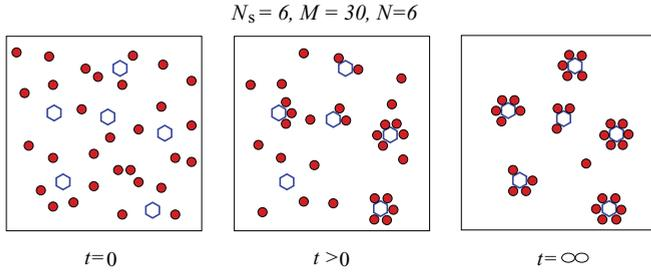
FIG. 1. (Color online) A heterogeneous nucleation process in which ligand monomers bind only to seeds. Here,  $N_s = 6$  seeds (open hexagons) are available to bind  $M = 30$  initial monomers (filled dots).
