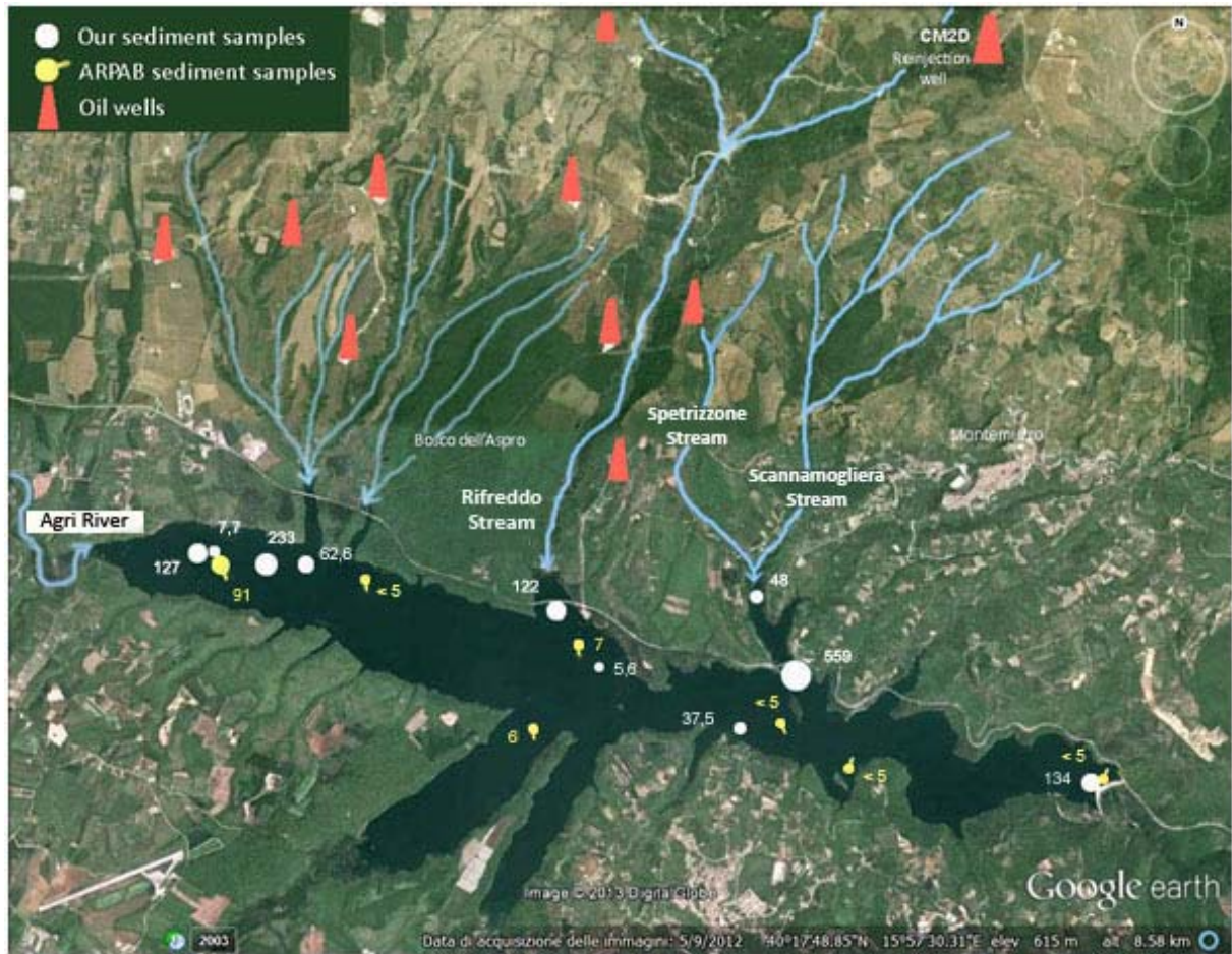
FIGURE 6 - Areal distribution of total hydrocarbons in subaqueous surface sediments of Lake Pertusillo. Dots show the location of our (white) and ARPAB's (yellow) sediment samples. The numerical values shown are concentrations of hydrocarbons in mg/kg. Courtesy of Google Maps.
