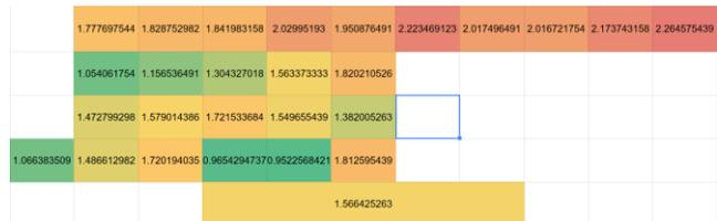
**Figure 9.** Heat map of the average lux readings for the numbers, letters, space bar, and left shift key. Colors reflect lux value, with red being larger and green being smaller.
