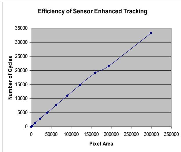
Figure 4. Computation cycles savings as the pixel area of the processing is decreased
