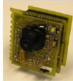
Figure 7. MicrelEye: Video Node Prototype
